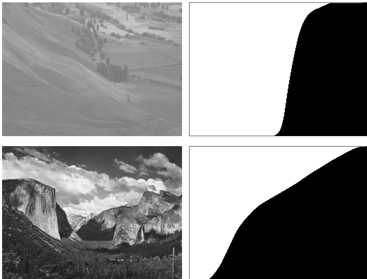
Figure 7: Comparison of cumulative histograms for a low contrast image (top) and a high contrast image (bottom). Lower contrast image tend to create a much sharper “wall” in the cumulative histogram, versus the more gradual increase in higher contrast images.
