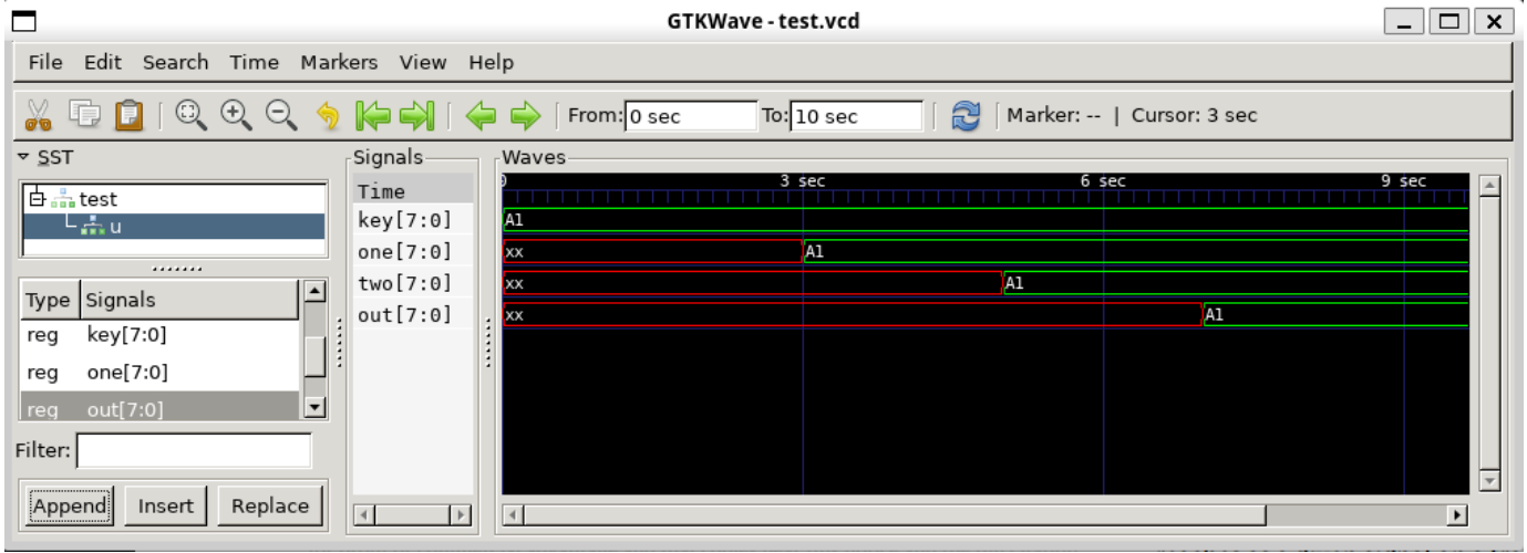
Fig. 1. The waveform of a design illustrating an information flow from key to out for which the path is ambiguous.
